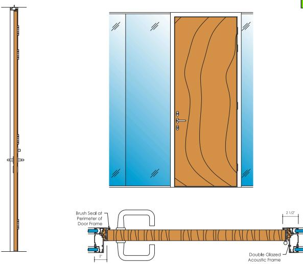
Timber Swing Doors are ideally suited for Conference Rooms, Offices or Other Spaces where a good sound insulation and reliability is required. They are compatible with most of the systems we offer which include: Solare™ Acoustic Double Glazed Partition System, Elevare™ Stacking Double Glazed High Wall System, Movare™ Movable Double Glazed Partition System or Transverto Monoblock™ Modular Wall Partition System.
